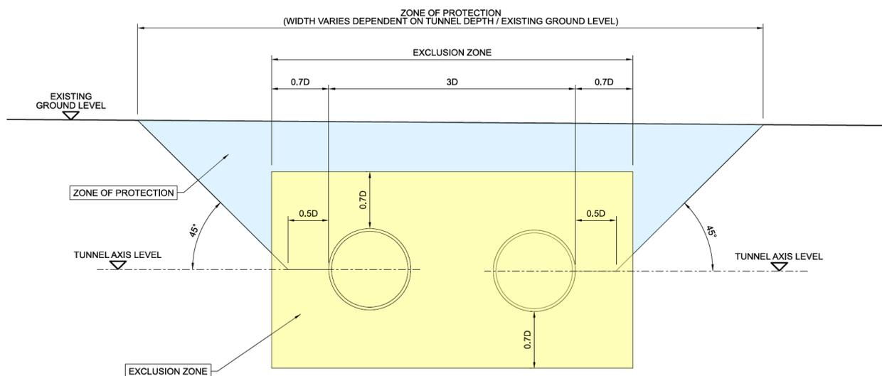
5.4.6 The Applicant would seek to impose restrictions on use the area identified as the first and second protection zones on the River Restriction Plans [[REP1-041](#)] to protect the tunnels. These restrictions are provided by Article 48 of the DCO. Further easements or restrictive covenants to protect the tunnels are not required.
